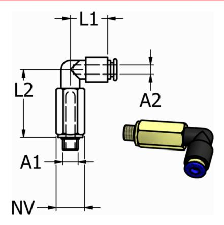
Ext. hose diameter A2 = 6 mm L1 = 32 L2 = 18.2 NV = 8 Thread A1 = M5
